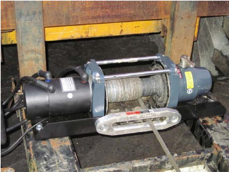
← A TDS-9.5c Goldfish winch fitted with a Bow '3' to a specially adapted and machined drum support
